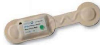
Fig 5. Wireless ECG sensor with separate transmitter and receiver. © Isansys Lifecare
