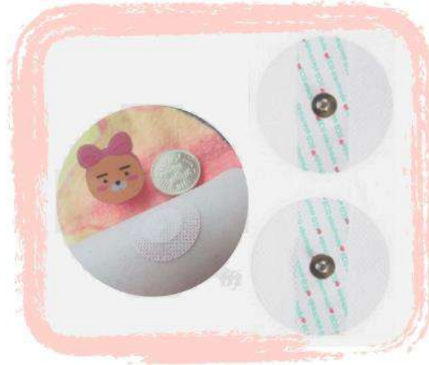
Fig 2. FIDES novel wireless ECG coin patch for multi purpose limb leads
